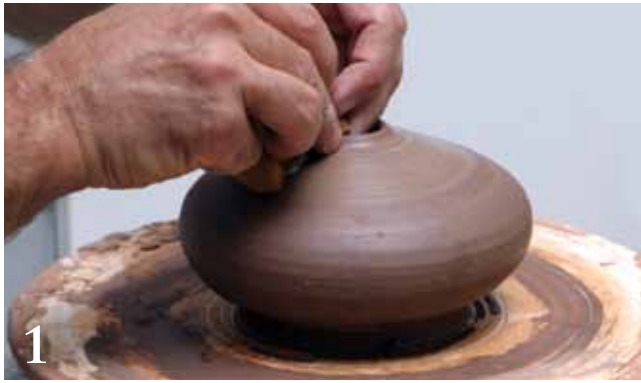
1 Throw the urchin form by bellying out then collaring in a cylinder and close it leaving only a small opening.
