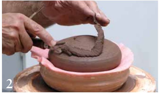
2 Place the piece upside-down in a padded chuck and then trim the bottom.
