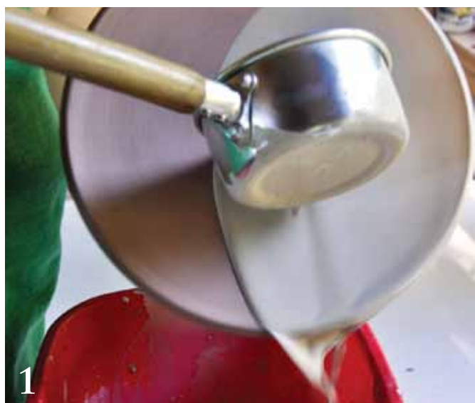
1 Pour white slip onto the middle of the plate, turning the piece clockwise until the entire face is covered.
